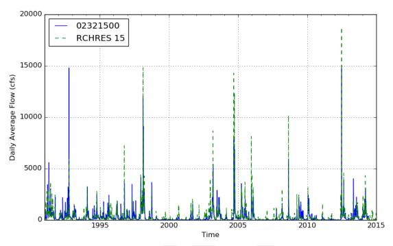
Figure 28. Example daily average observed (02321500) and modeled (RCHRES 15) calibration plot for the Santa Fe River Gauge at Worthington Springs.
