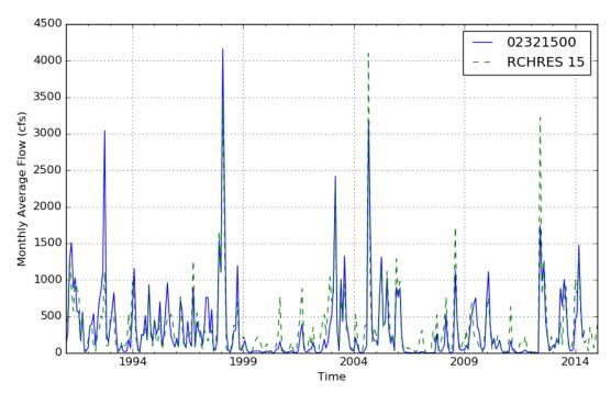
Figure 27. Example monthly average observed (02321500) and modeled (RCHRES 15) calibration plot for the Santa Fe River Gauge at Worthington Springs.
