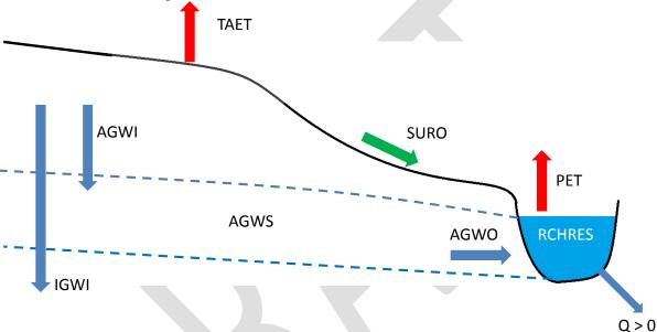
Figure 18. Conventional representation of a sub-watershed for a tributary basin.
