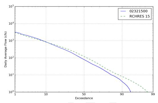
Figure 28. Example frequency distribution curve for observed (02321500) and modeled (RCHRES 15) daily average flows over the period of record for the Santa Fe River Gauge at Worthington Springs.
