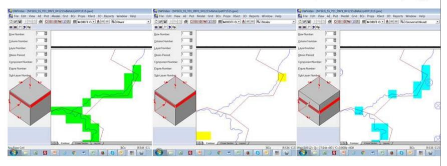
Layer 1 has a River node and Drain node in the same cell (at the location of a spring) with the same head assignment.
