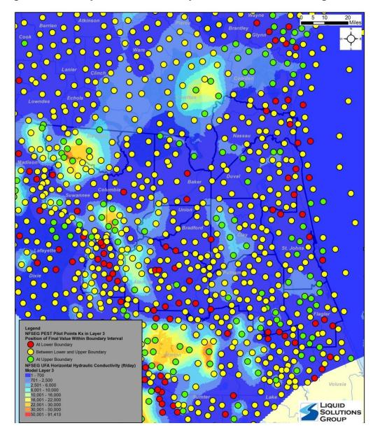
Figure 13 - UFA Hydraulic Conductivity and PEST Pilot Point Ranges
