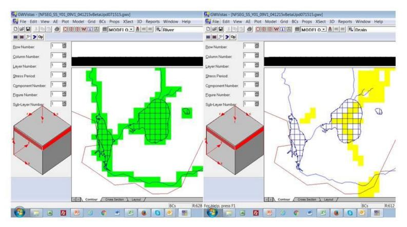
Multiple Drain nodes with area of River nodes representing Lake Lockloosa. The River node assigned heads can be > or < the Drain node assigned heads.
